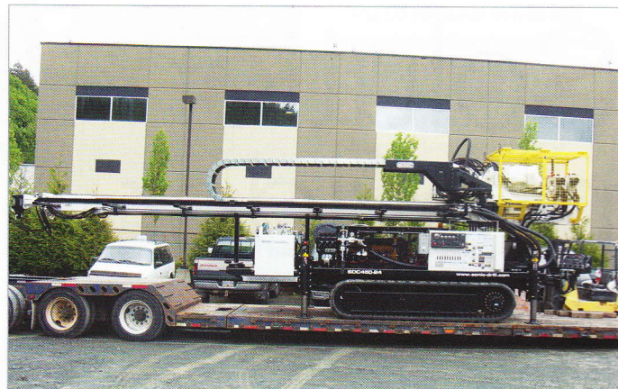
Geomechanics' new Sonic 450-24 is said to bore five times faster than conventional rigs
