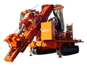
The safety cage has a hinged access door on the front and opening the access door immediately stops the spindle rotation. Drillers can also activate a spring-centered override switch at the console which enables 5 rpm of rotation at low torque. Closing the door reactivates full rotation and torque. All switches and circuits are designed to be tamper-proof so that operators cannot bypass the safety system.
