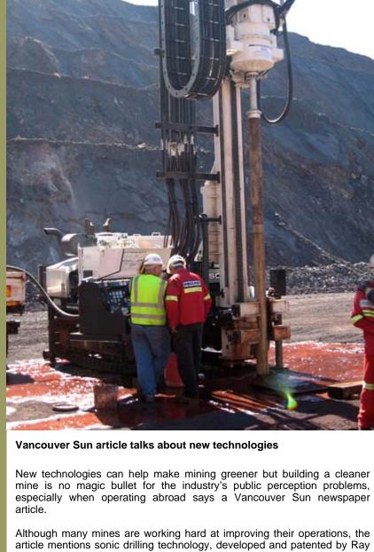
Roussy and manufactured by the Sonic Drill Corporation, as a positive step forward for the industry. MiningWatch Canada's Ramsey Hart can see the benefits of sonic drilling. "They don't need to use drilling muds or fluids, the materials that are put down with the core drill to provide lubrication to get the rock material out of the hole," he said. "Managing those drilling muds is always an
