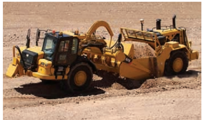
COMPUTERS ON BOARD: Today's H-series scrapers are loaded with custom software to improve accuracy and efficiency.
