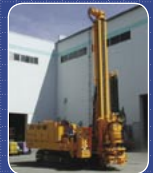
SONIC CRAWLER RIG
