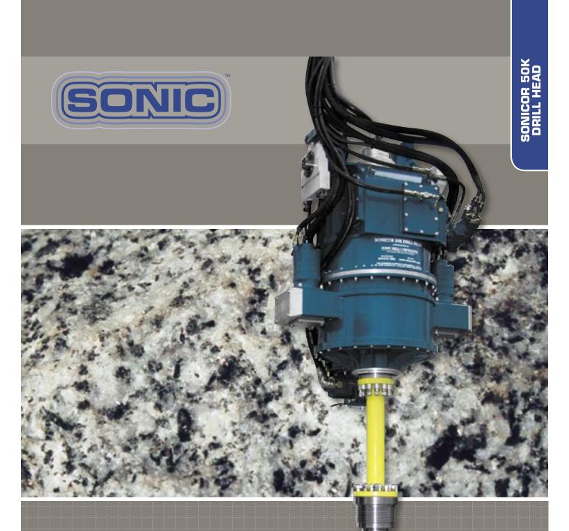
The **SONICOR 50K** sends high frequency mechanical oscillations down the drill string to the bit. The operator controls frequencies to suit specific conditions of soil/rock geology. High frequency vibrations fluidize the soil particles at the bit face, allowing for fast and easy penetration in most geological formations, including boulders and bedrock.
